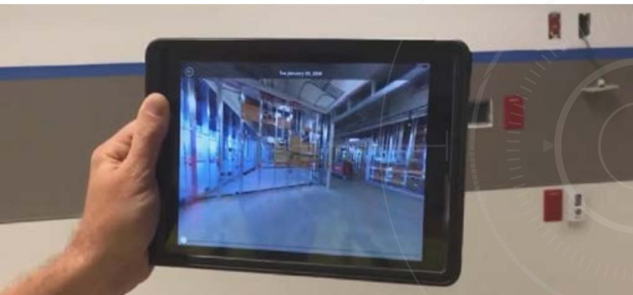
Doxel and other 3D-imaging tools use video capture to track progress and identify errors. A project team member wearing a camera walks the jobsite to document construction progress and capture a comprehensive scan of recent installations. Once the worker completes the site walk, they upload the data and the software measures progress based on the project schedule and its building information model.
